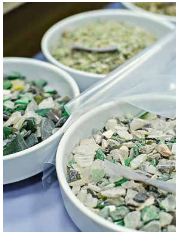
At the IGR, cullet mixtures are examined to determine how the mixture affects further processing into recycled glass
