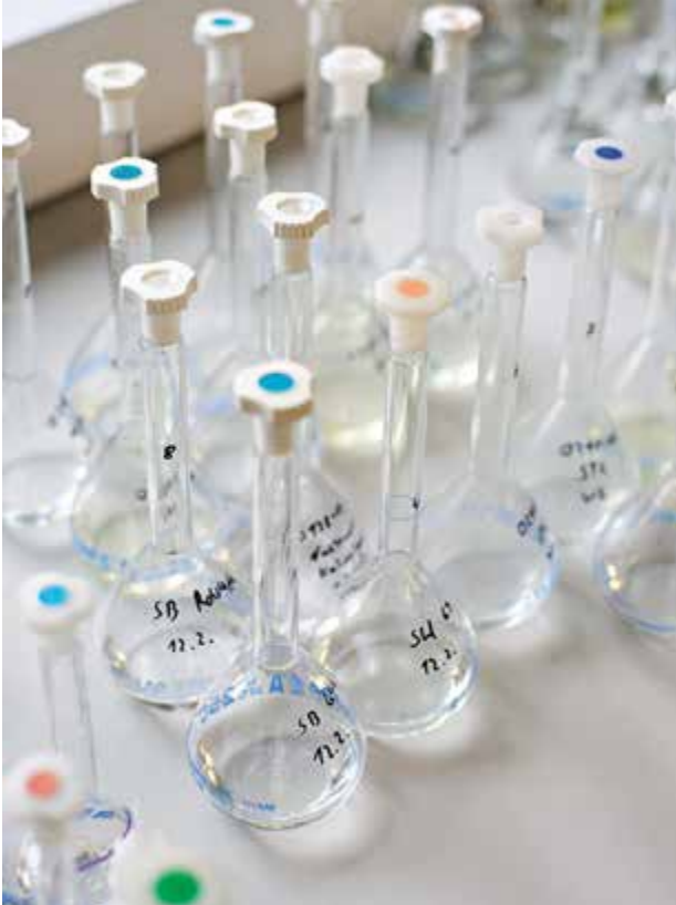
Before the actual measurement series starts in the laboratory, sample solutions are prepared in volumetric flasks
